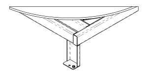
STRUCTURAL CHANNEL WELDED RISERS FOR ELEVATION UP TO 20" (JACK-BOLT SUPPORTS FOR TALLER ELEVATIONS)
