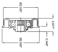
MAX SPEED: 200 RPM LOAD RATING: 145 LBS.
