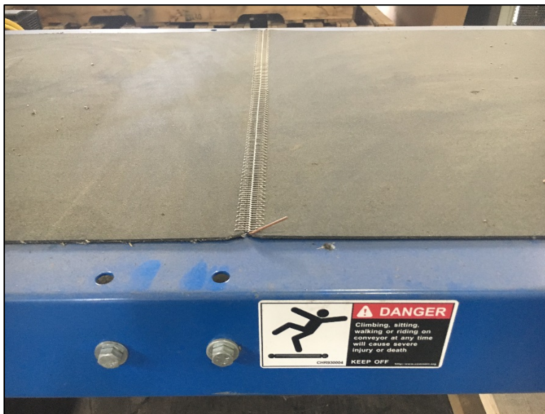
Figure 4 – Belt Ends Laced Together on Top of Conveyor
