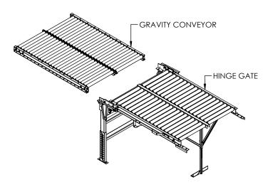
WHEN USING WITH GRAVITY CONVEYOR, NO INFEED IS REQUIRED.
