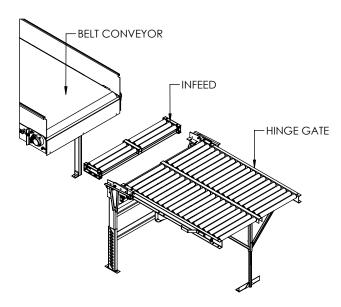
WHEN USING WITH BELT CONVEYOR, INFEED IS REQUIRED. CUSTOMER IS RESPONSIBLE FOR CONNECTION. FIELD WELD MAY BE REQUIRED.
