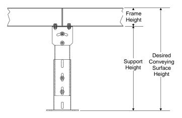
Figure 2.1 – Support Height Adjustment
