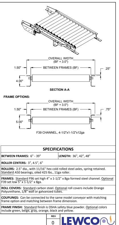
Model: HS2511 - Spring Assisted Hinge Gate, 2.5 diameter roller 11 guage
